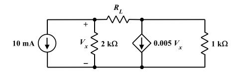
What value of  $R_L$  will absorb maximum power from the remainder of the circuit?
